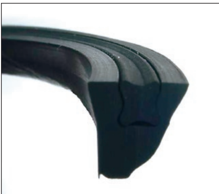
Fig. 2-7. Instability failure of a square profile piston seal
