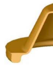
"D" Bead - Under Worse resistance to trapping air Worse flow for less knit lines Worse flash location for trimming
