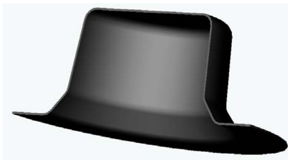
Figure 7 – A Typical Double Taper Diaphragm
