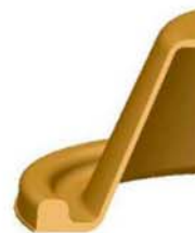
"D" Bead - Over Worse resistance to trapping air Worse flow for less knit lines Better flash location for trimming
